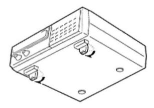
To more easily view the keyboard and display, elevate the front of the scanner by unfolding the front feet.
