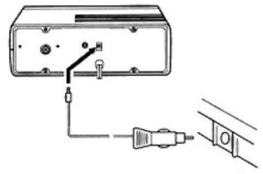
You can power your scanner from your vehicle's cigarette lighter socket by using a DC Adapter (not supplied). The vehicle must have a 12-volt, negative ground electrical system.
