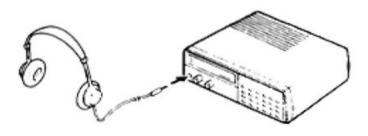
Note: Plugging in headphones automatically disconnects the internal speaker.
