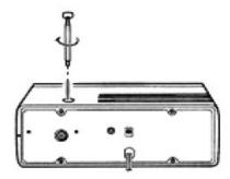
To attach the supplied telescoping antenna, simply screw it into the hole on the top of the scanner.
